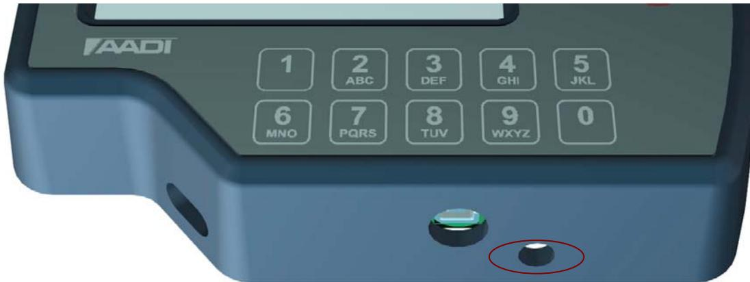
**Figure 1-1** The Calibration Switch is placed underneath the Main Unit.
